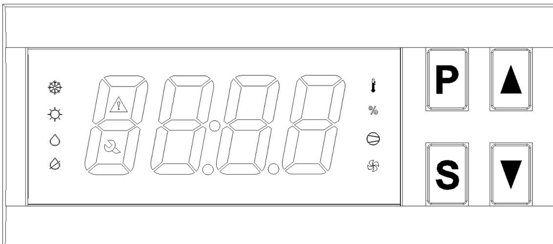
Eco mode: The brightness of display will reduce when no key operation for 30 seconds.
